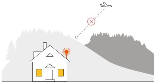
Bad position – hills blocking antenna
