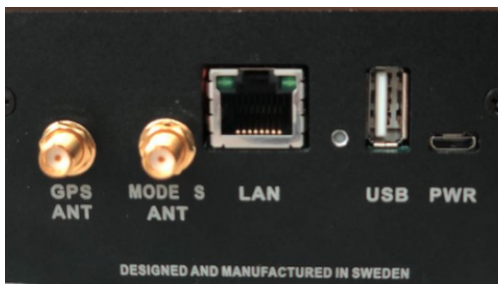
Rear view of the Flightradar24 receiver with the available connections
